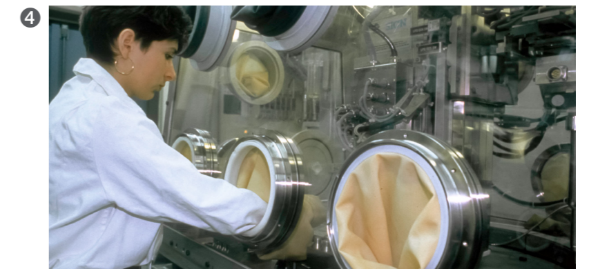
AD gloves mounted on ejectable rings
